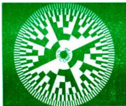
Photo A—Discs used in Stroboconn.
